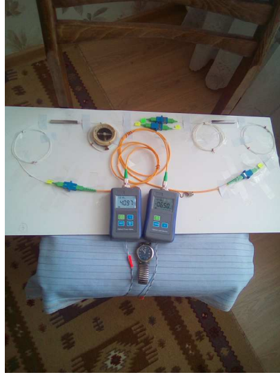
FIG. 2, Experimental Set-up with a hybrid Mach-Zender interferometer and light source with Fabri-Perot laser diode.
